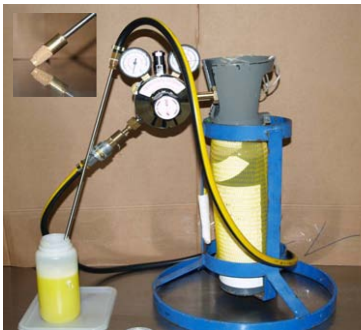
Figure 2.15: Metallic frit and rod setup used for sparging the sample prior to aeration.
