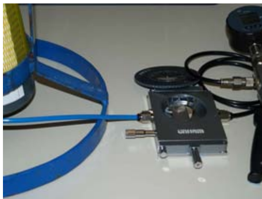
Figure 2.14: Pressure cell setup with a dedicated gas line attached to the chamber via the blue flex-hose. The image also shows the quartz crucible that holds the sample. The Black hose and pressure gauge are there for the pressure read-out.
