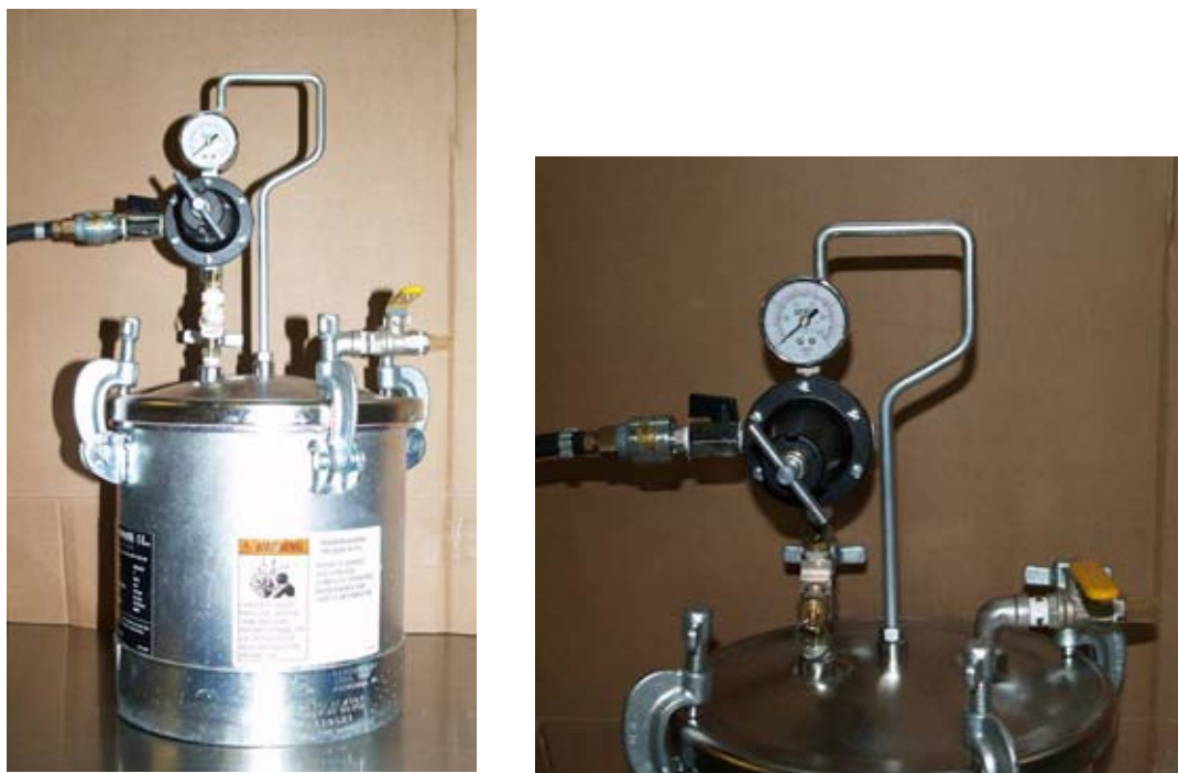
Figure 2.12: Binks Pressure pot. Capable of pressures up to 10 bar absolute.
